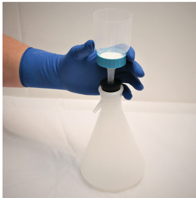
Photo 2 Set the blue base of the filter funnel onto the clear filtration stem you placed into the #8 one-hole stopper on top of the filtration flask.
